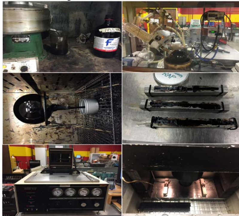
Figure 30. Test Procedure for BBR
